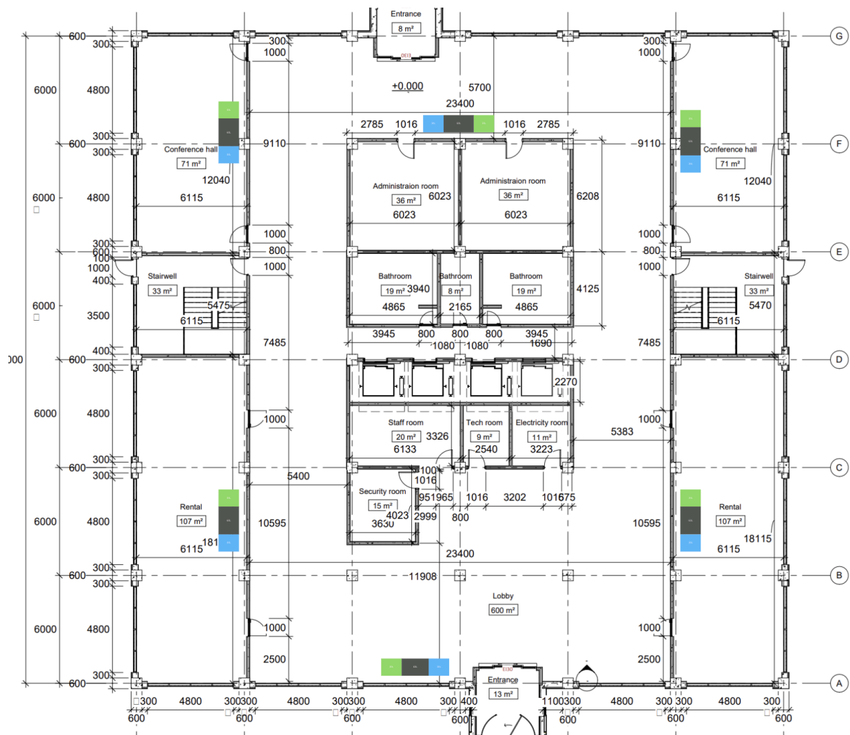
Figure 5.3. Ground floor waste station placement.
