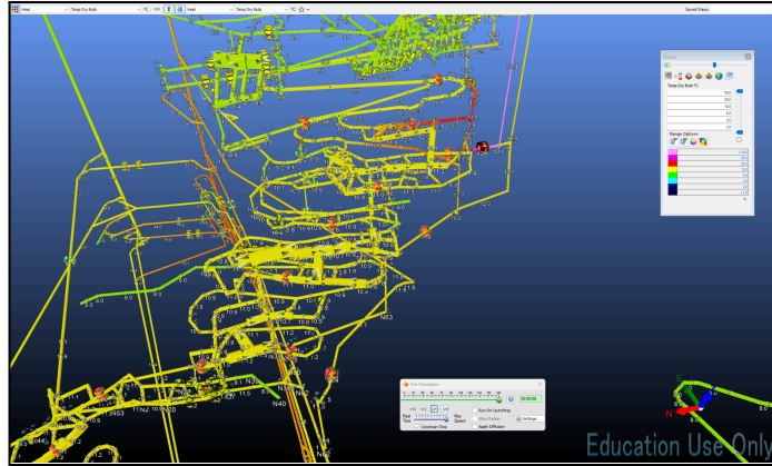
Figure 42. Heat distribution after fire simulation with fan failure (Scenario 3).
