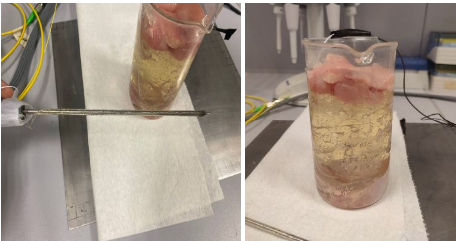
Figure 4.1: A) Shape sensing needle; B) chicken meat and gelatin-based phantom
