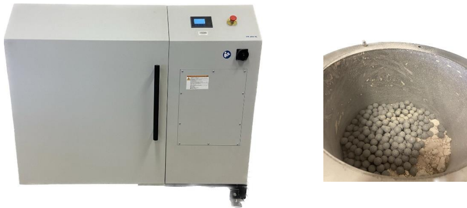
Figure 24: Balling mill for metakaolin
