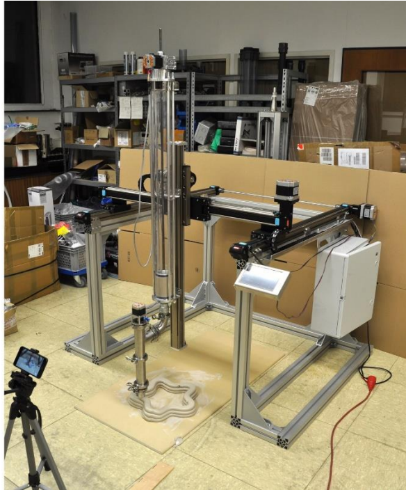
Figure 47: Concrete 3D printer
