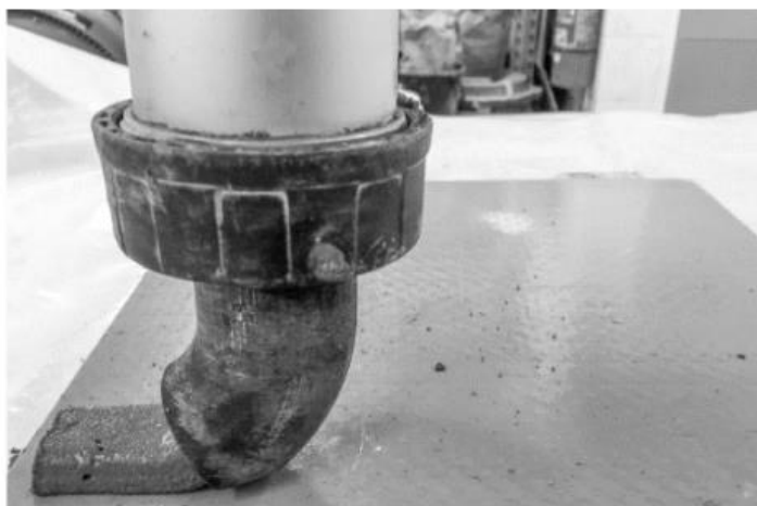
Figure 16: Nozzle with a 45-degree angle on its rectangular opening [69]
