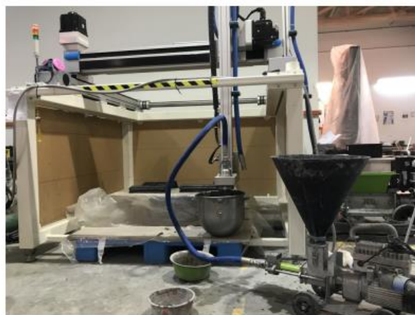
Figure 15: Gantry printer used by Lao et al. [65]
