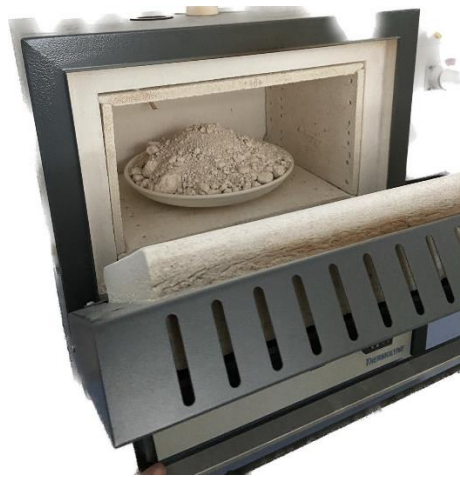
Figure 23: Furnace for kaolin
