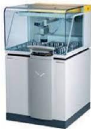
Figure 22: XRF Axious Max [129]
