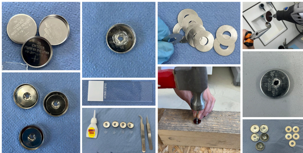
Figure 7. Illustration of preparation of “home-made” cell for Raman Spectroscopy
