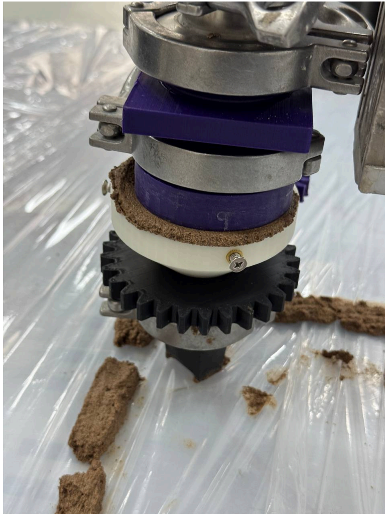
Figure 22: Detachment of lower from upper adapter
