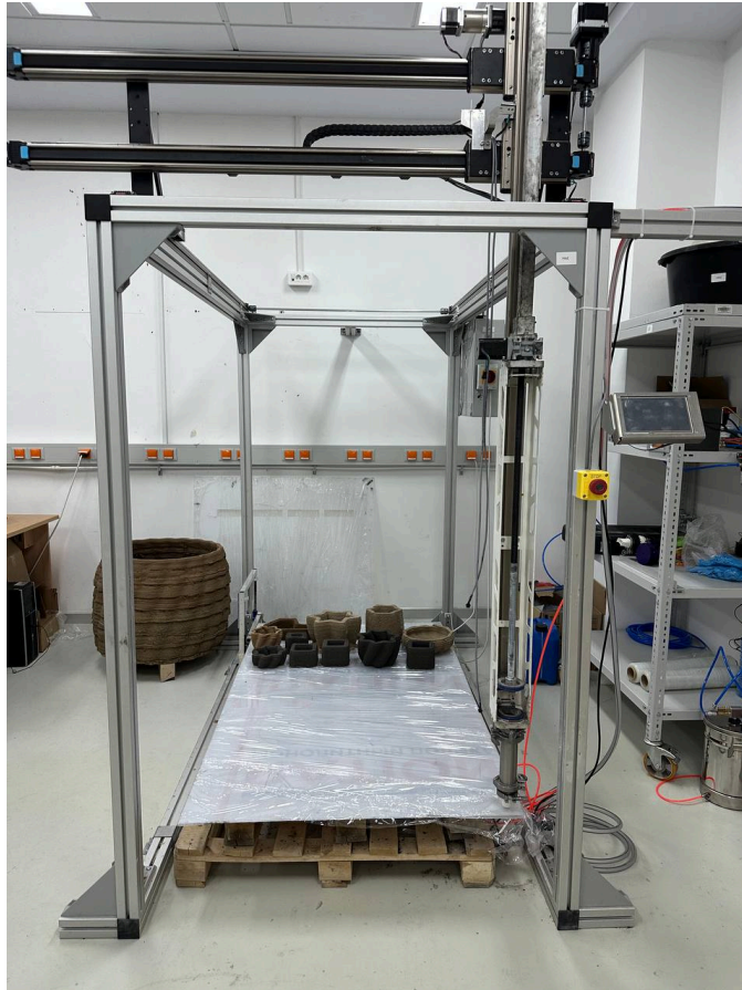
Figure 1: Concrete printer in NU
