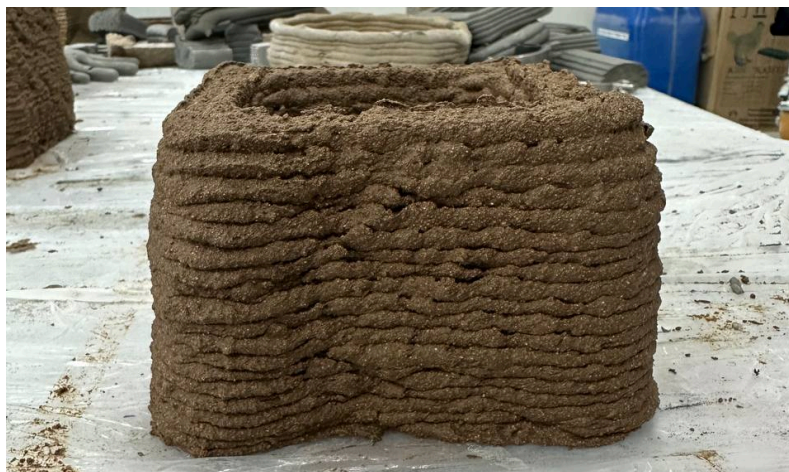
Figure 28: The print with geopolymer with sand:clay ratio of 137:45
