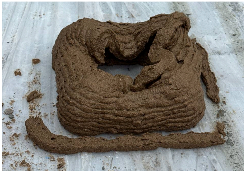
Figure 26: The print with geopolymer with sand:clay:water ratio of 125:45:6
