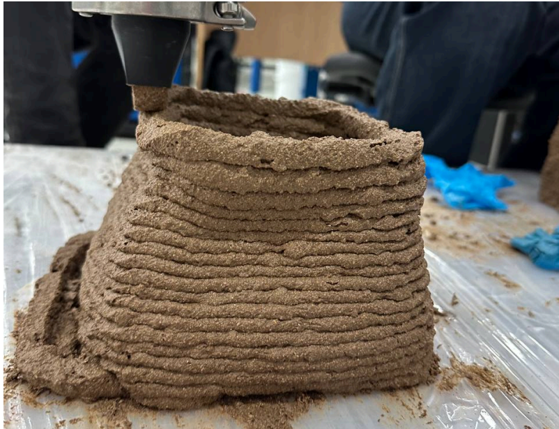
Figure 27: The print with geopolymer with sand:clay:water ratio of 137:45:6
