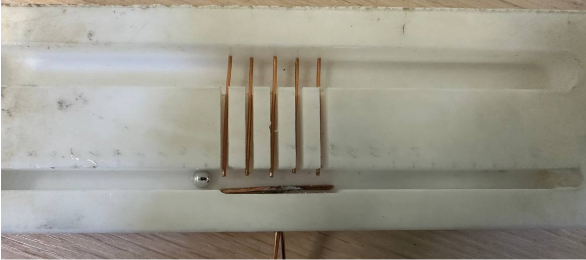
Figure 3.1: Copper elements and fluid drop of the Galinstan installed in the mold.
