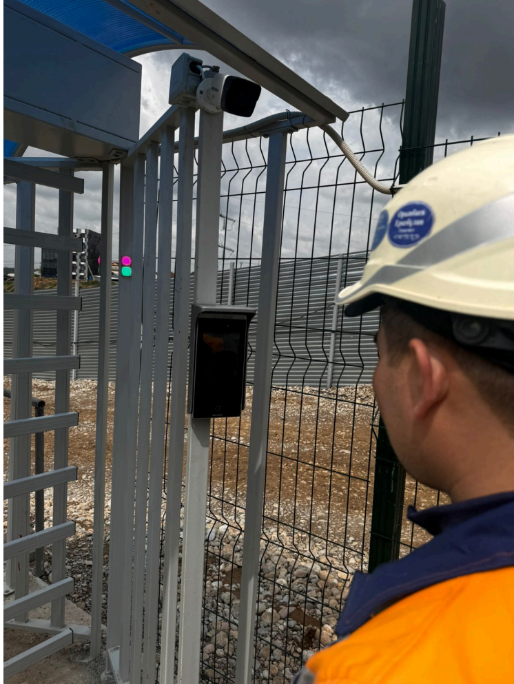
Figure 5.30. Face identification for safety gear
