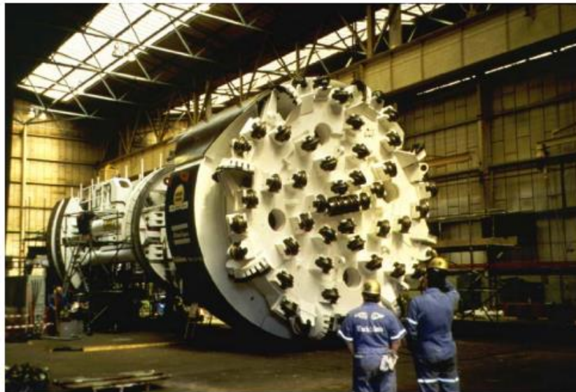
Figure 3.1. High Power TBM utilized for the Queens Fresh Water Transfer Tunnel (Yagiz, 2002)
