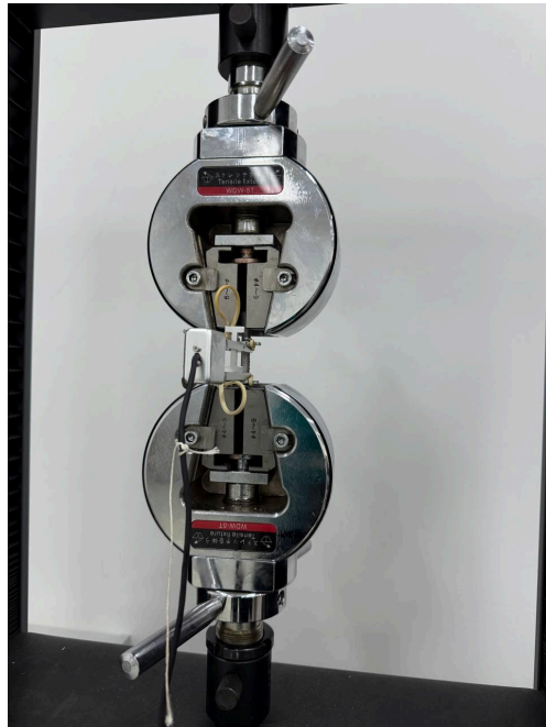
Fig. 11 Sample on WDW-5T machine
