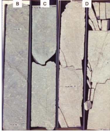
Figure 8. Examples of fractured core samples (Warrlich, et al., 2010)
