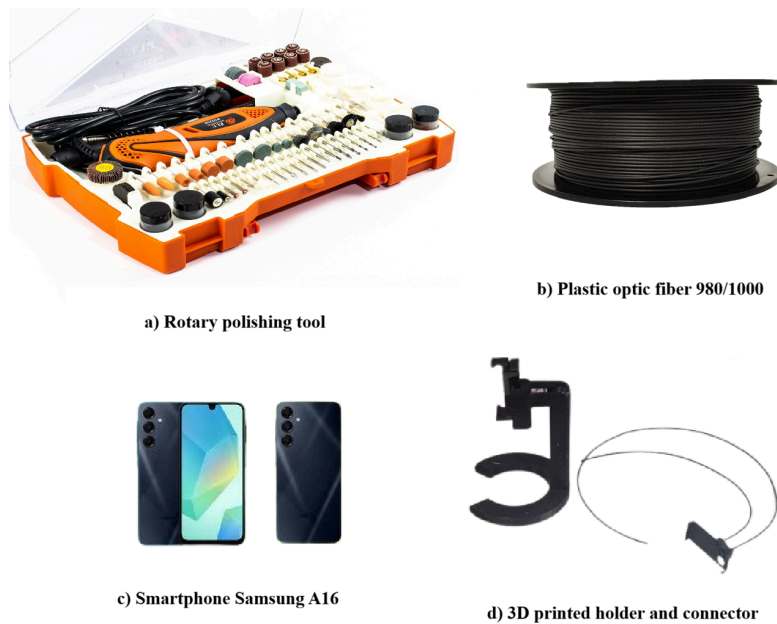
Figure 3-1: Materials used for fabrication and calibration stages.
