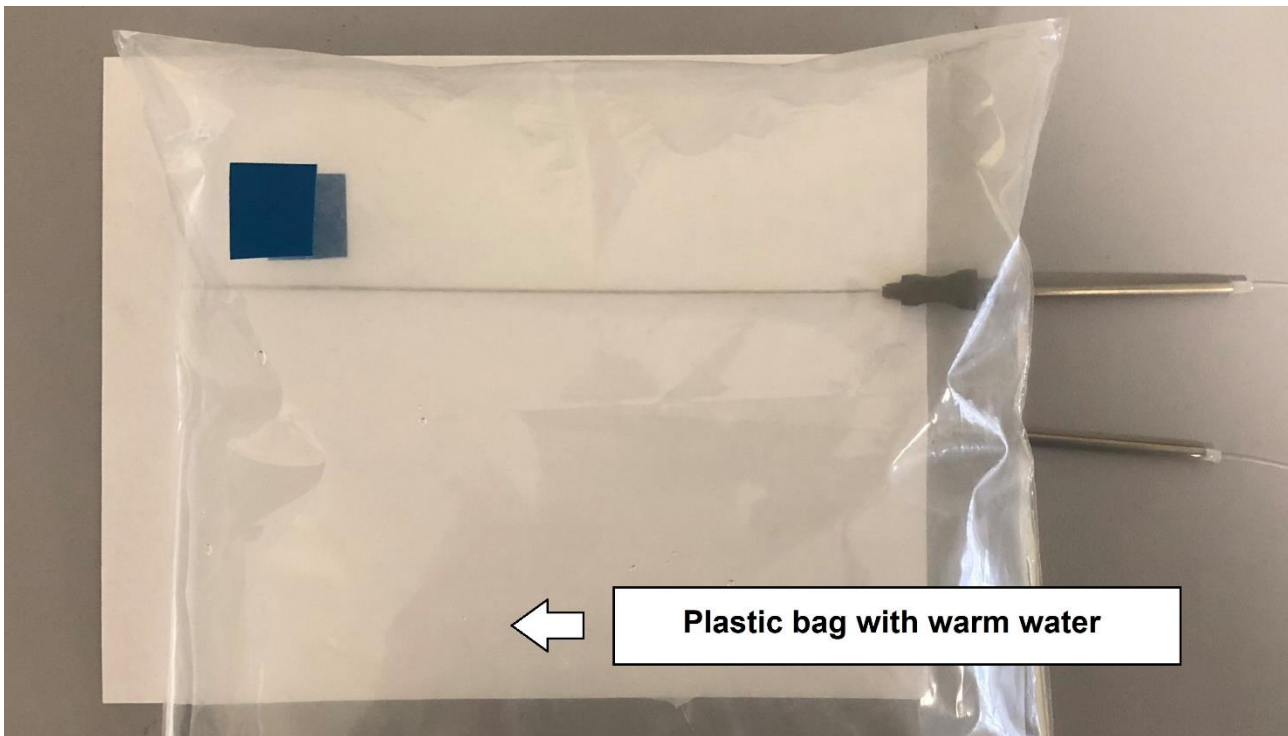
Figure 3.3.2: Placing a plastic bag with warm water on top of the fiber-optic sensors to observe the effect of a catheter on the temperature change
