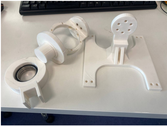
Figure 4.16: 3D printed Upper Body parts
