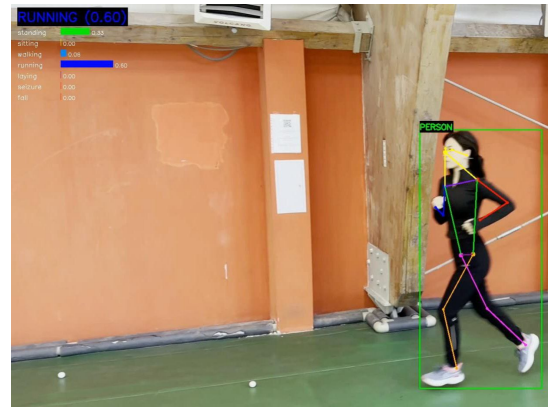
(a) Visualization of the system detecting a 'Running' activity, including pose estimation and confidence scores.
