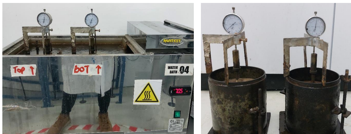
Figure 3.9: Expansion procedures for stockpiled BOF slag
