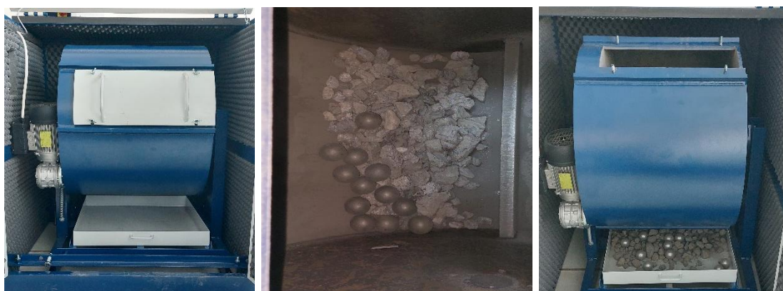
Figure 3.5: Los Angeles abrasion test on stockpiled BOF slag.
