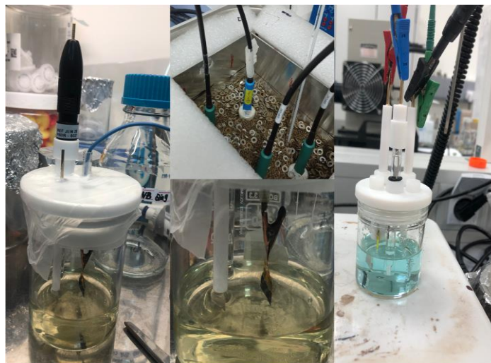
Figure 6.9. The bioelectrochemical cell is assembled with a polymer film.
