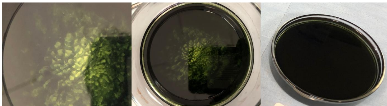
Figure 4.8. The initiation, propagation, and termination phases of the polypyrrole film formation process.
