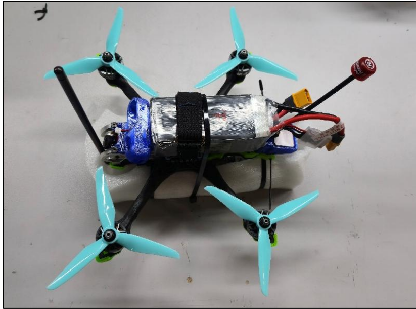
Figure 4.1: UAV platform with SDR receiver payload
