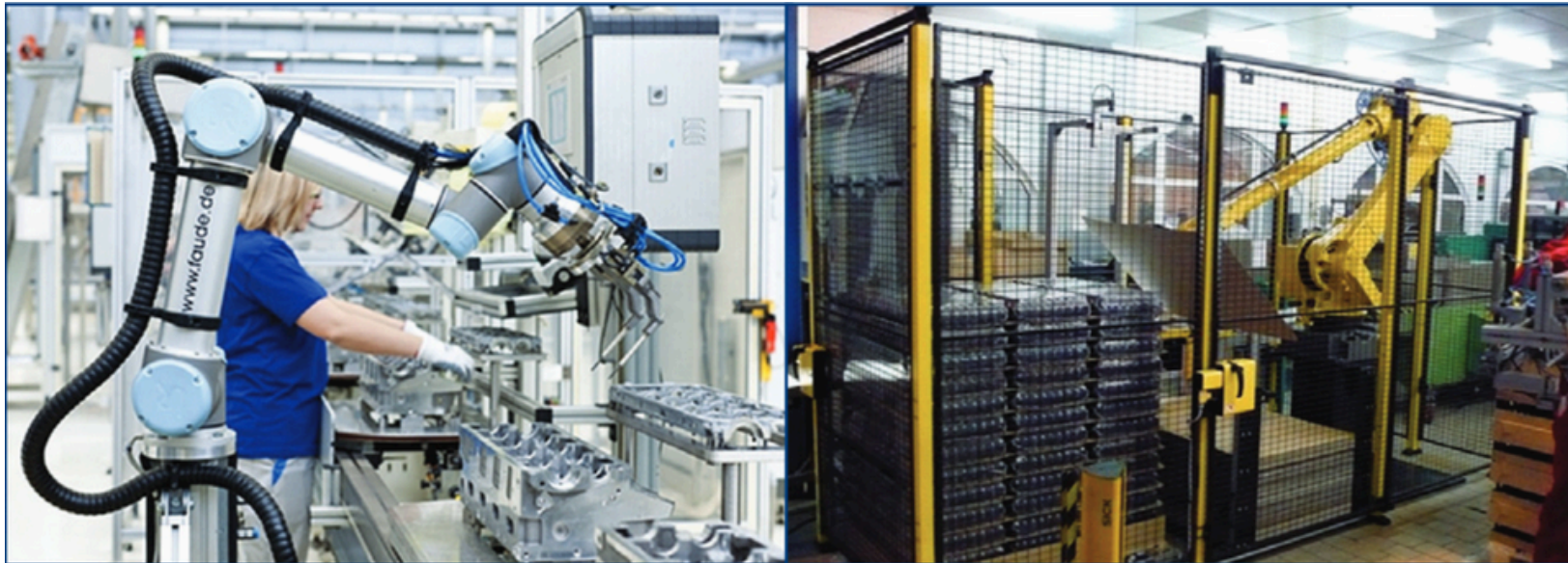
Figure 1. Robot workplace with collaborative (left figure) and traditional industrial robot (right figure) (Vysocky, A. L. E. S., & Novak, P. , 2016)
