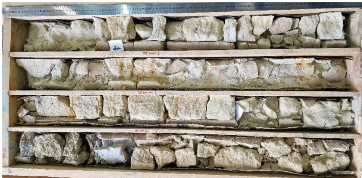
Figure 7. Example of historical core material used for sedimentological description in South Tortkuduk, illustrating the unconsolidated character of the reservoir and the preservation challenges of the core dataset. (Smagambetov et al., in preparation).
