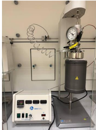
Figure 15. Batch reactor experiment setup.
