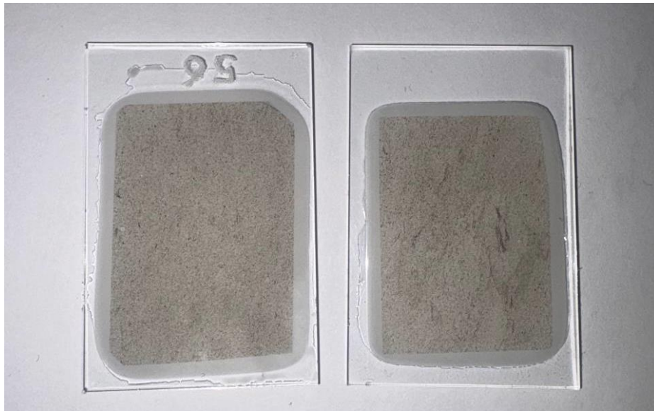
Figure 14. Thin Sections prepared from the core plug. Before the reaction (left) and after the reaction (right).
