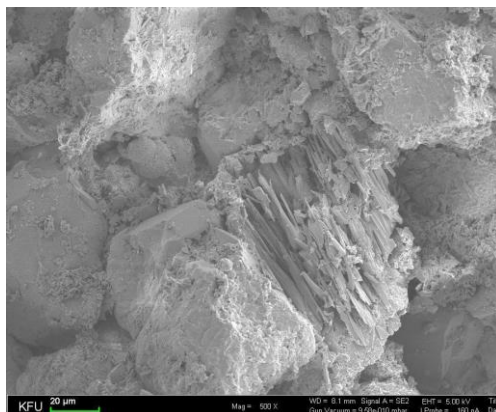
Figure 26. Grains of corroded feldspar.
