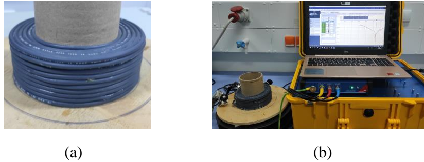
Figure 4.7. Test equipment: (a) fabricated winding; (b) winding FRA measurement
