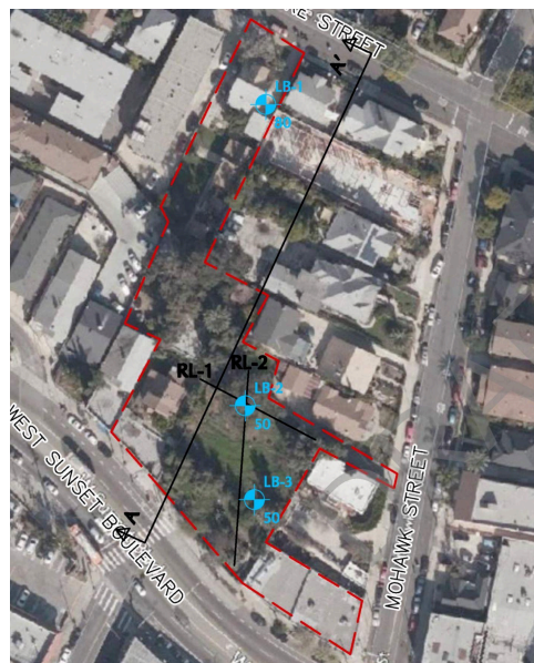
Figure 4.1. Approximate boreholes' location
