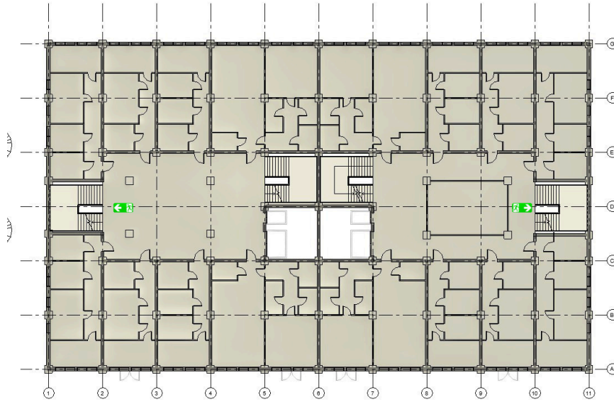
Figure 2.21. Emergency evacuation plan of residential floors.
