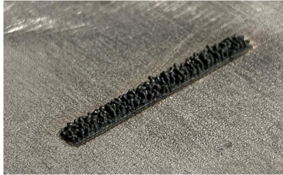
Figure 10.2 Inconel 718 specimen with unexpected defect formation
