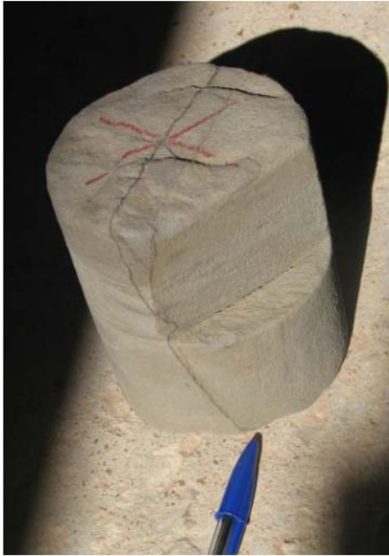
Figure 12. Fracture studies: (left) Mineralized fracture from well KB-2 core, (right) Fracture azimuth from FMI image log in well KB-502 (Iding & Ringrose, 2009)
