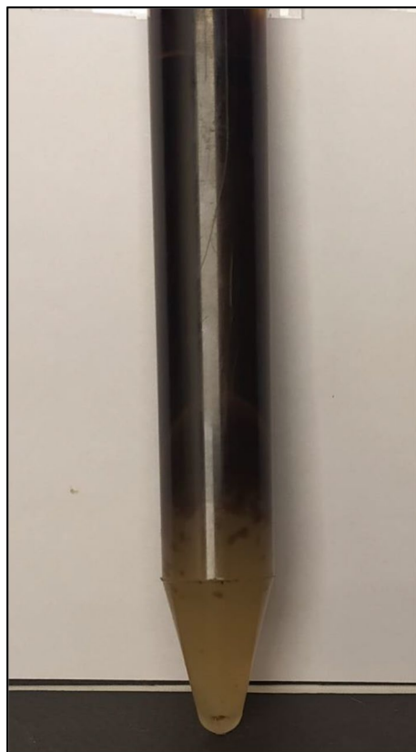
Figure 6. Separation of two phases in the centrifuge.
