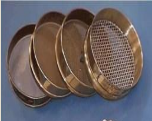
Figure 5. Grain-Size Analysis: ASTM D422-63
