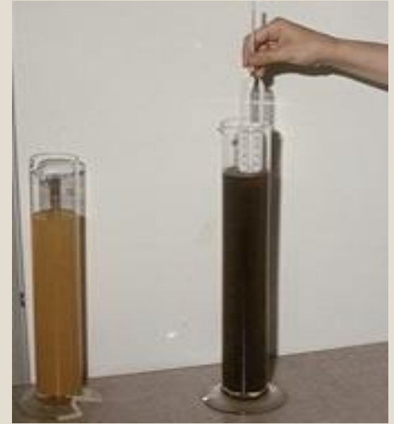
Figure . 7 Hydrometer analysis ASTM D7928-21e1
