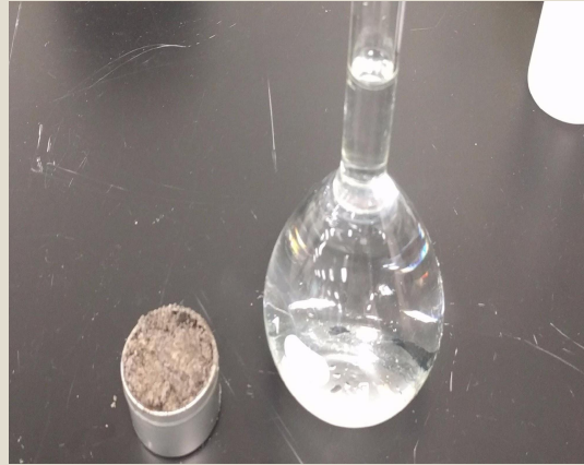
Figure 6. Specific gravity Test: ASTM D854-06
