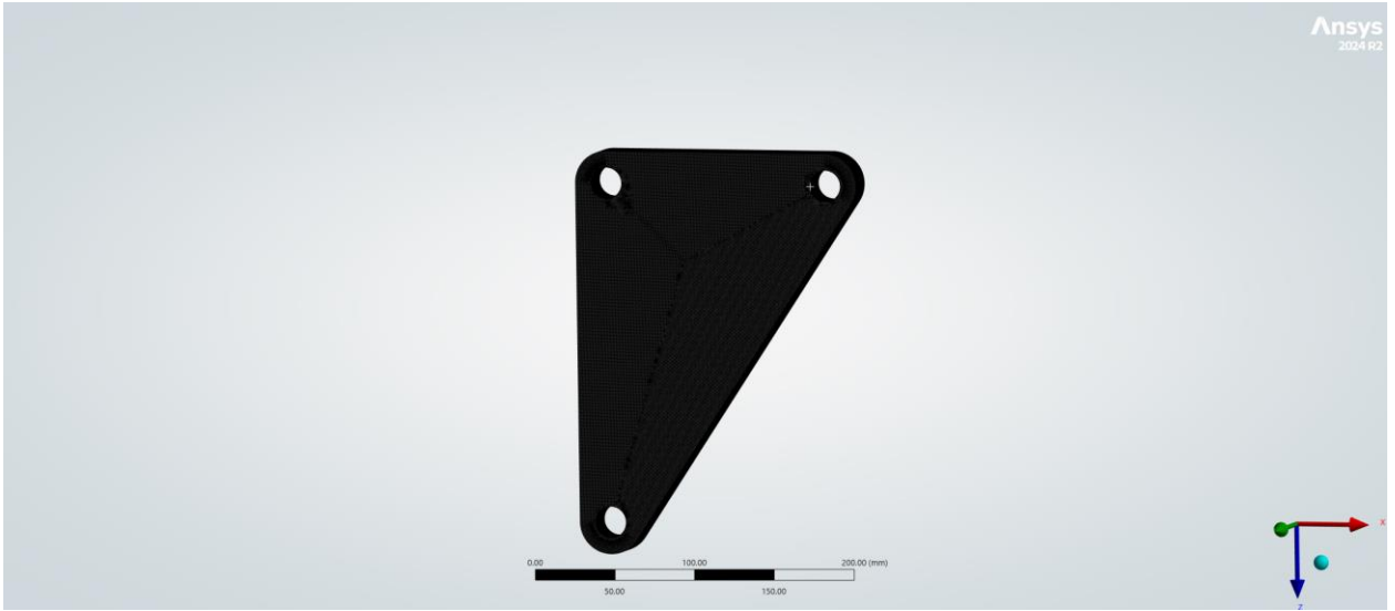
Figure 6.2 The final mesh of the model with a 0.7mm element size
