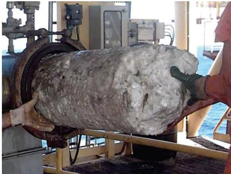
Figure 1. Gas hydrate plug recovered from a subsea pipeline (Koh et al. 2011)
