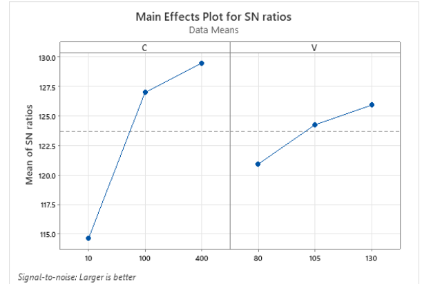
Figure 5.2: S/N response for MRR for \mu -EDM for Ti-29Nb-13Ta-4.6Zr.
