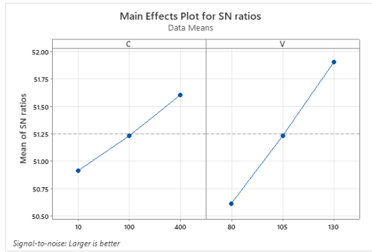
Figure 5.13: S/N response for surface microhardness for \mu -WEDM for Ti-35Nb-7Zr-5Ta.
