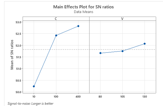
Figure 5.14: S/N response for surface microhardness for \mu -WEDM for Ti-29Nb-13Ta-4.6Zr.
