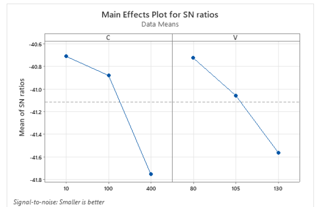
Figure 5.16: S/N response for kerf width for \mu -WEDM for Ti-29Nb-13Ta-4.6Zr.
