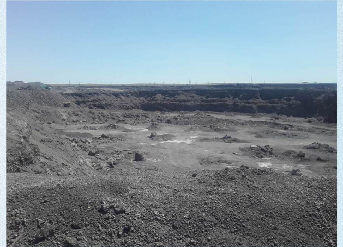
Fig 5. Basic Oxygen Furnace Slag (BOFS) stockpile at JSC "ArcelorMittal Temirtau" site, Kazakhstan.
