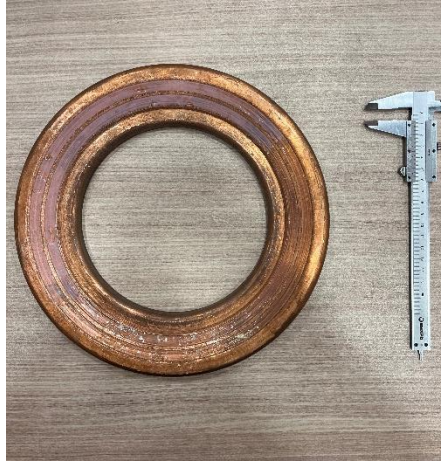
Figure 3. 2 grooved anode filled with liquid dielectric
