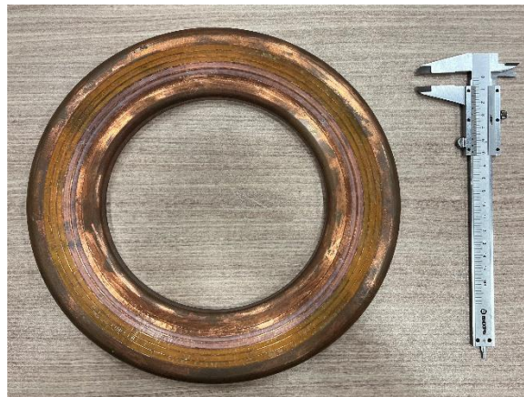
Figure 2. 4 grooved anode filled with liquid dielectric
