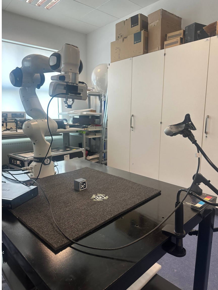
Figure 2: The real robot setup, the Franka Panda arm, the table workspace, the object with AprilTag on top, the goal position marker, and the overhead Intel RealSense camera mounting.
