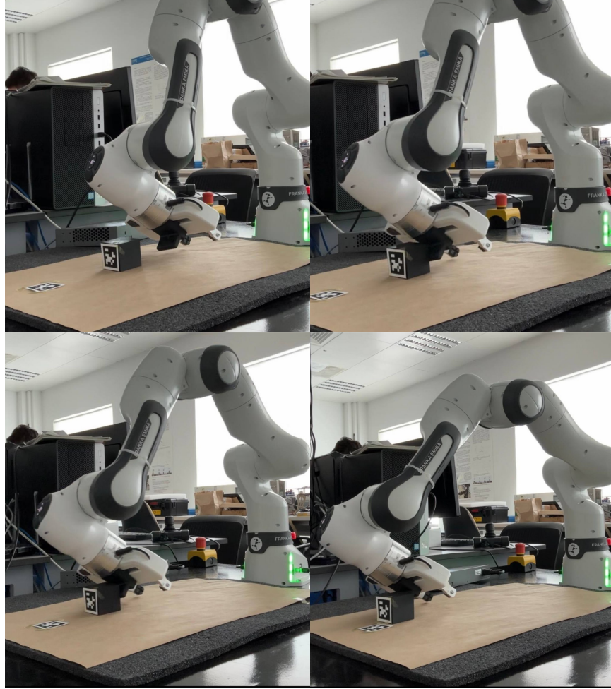
Figure 9: A sequence of 4 frames from a successful straight-line episode. Frame 1: initial state with cube at approximately x=0.45 , arm at home position. Frame 2: arm completing its approach arc to position behind the cube. Frame 3: arm in contact with cube mid-push. Frame 4: final state with cube close to the goal marker.
