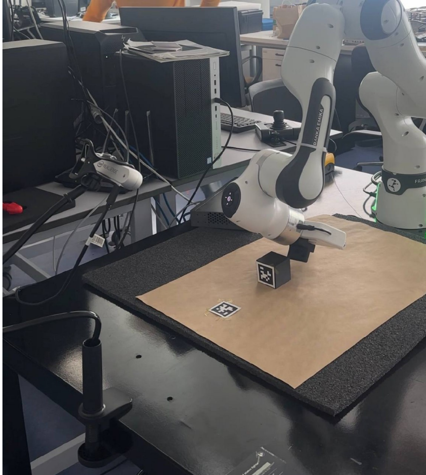
Figure 8: Photo of the complete real robot setup with the Franka Panda arm over the workspace, the black cube with AprilTag on its side face placed on the craft paper surface, the flat goal marker on the table, and the overhead Intel RealSense D435 camera.
