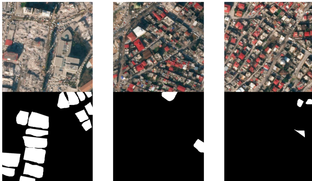
Figure 8. Example of original and masked version of collapsed buildings (Haciefendioğlu et al., 2023)
