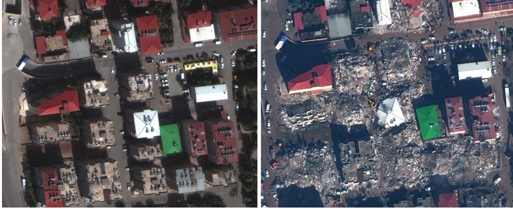
a) b) Figure 15. Satellite imagery of a) pre-earthquake and b) post-earthquake for Adiyaman The border lines of rubbles (or collapsed building areas) were marked using Polygon function in ArcGIS as in Figure below:
