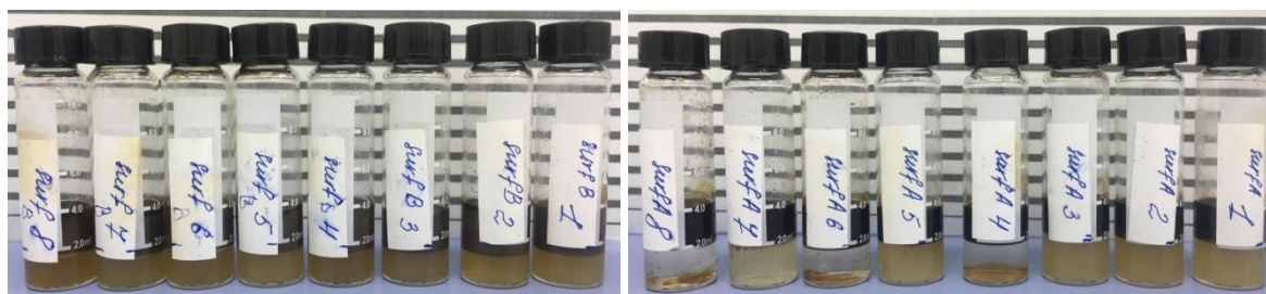
Figure 24. a. phase behavior for surf B (Soloterra 113H) after 3 days at 80°C in the left side b. phase behavior for surf A (XOF-26S/314C in 70/30 ratio) after 3 days at 80°C in the right side
