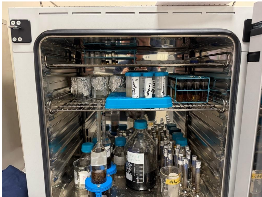
Figure 18. The placement of polymer solutions in vials inside of the heat oven with temperature of 63°C.
