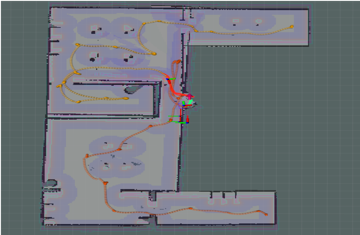
Figure 4.6: Exploration completion and map merging for two turtlebots
