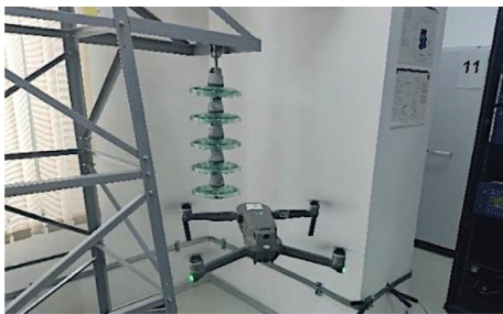
FIGURE 10: UAV-based insulator image collection.
