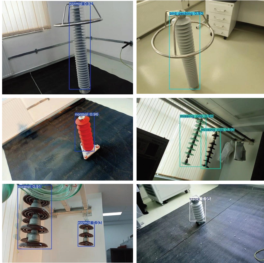
FIGURE 8: Detection and classification of insulator mechanical damage using YOLOv8l on the test set.
