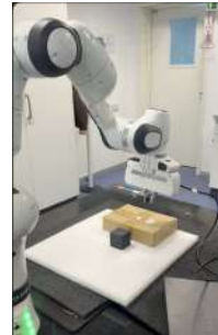
Figure 5-4: Task: “Pick up the black cube and put it on the box.” The robot descends the end-effector to the grasp pose, closes the gripper to secure the cube, and transports it to the target plate. After placing the object, the end-effector returns to the home position.
