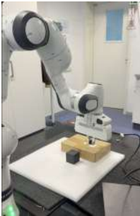
Figure 5-4: Task: “Pick up the black cube and put it on the box.” The robot descends the end-effector to the grasp pose, closes the gripper to secure the cube, and transports it to the target plate. After placing the object, the end-effector returns to the home position.
