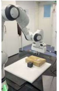
Figure 5-4: Task: “Pick up the black cube and put it on the box.” The robot descends the end-effector to the grasp pose, closes the gripper to secure the cube, and transports it to the target plate. After placing the object, the end-effector returns to the home position.
