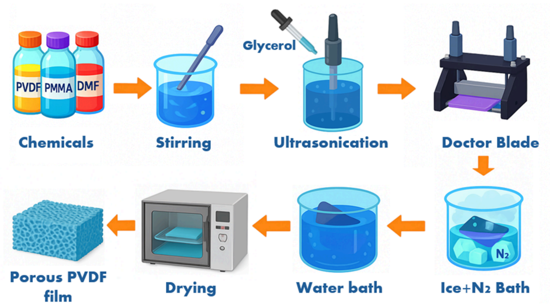
Figure 6. Preparation of PVDF film.
