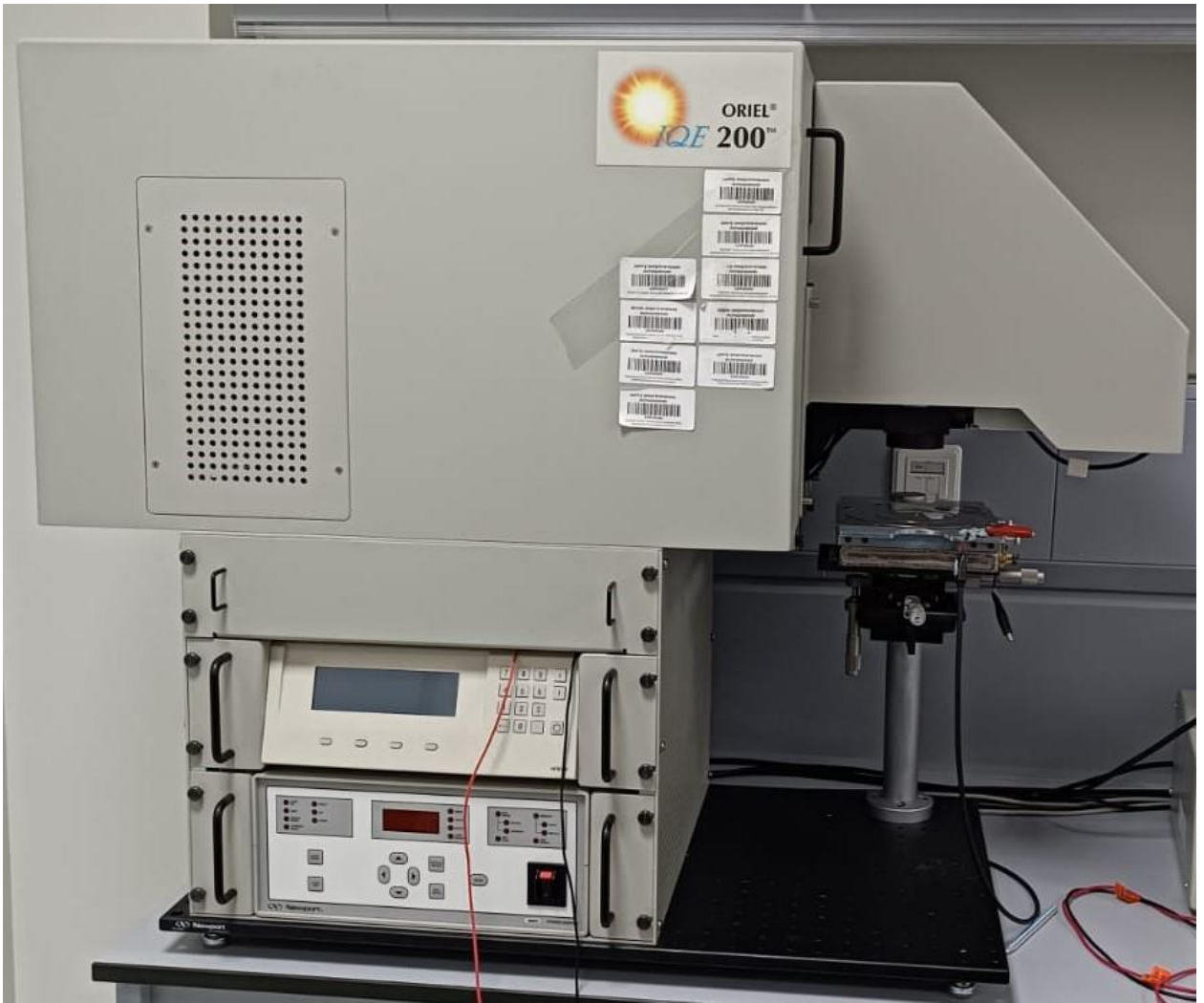
Figure 3.12: A photographic image of the EQE setup used for the PSCs in the presented work
