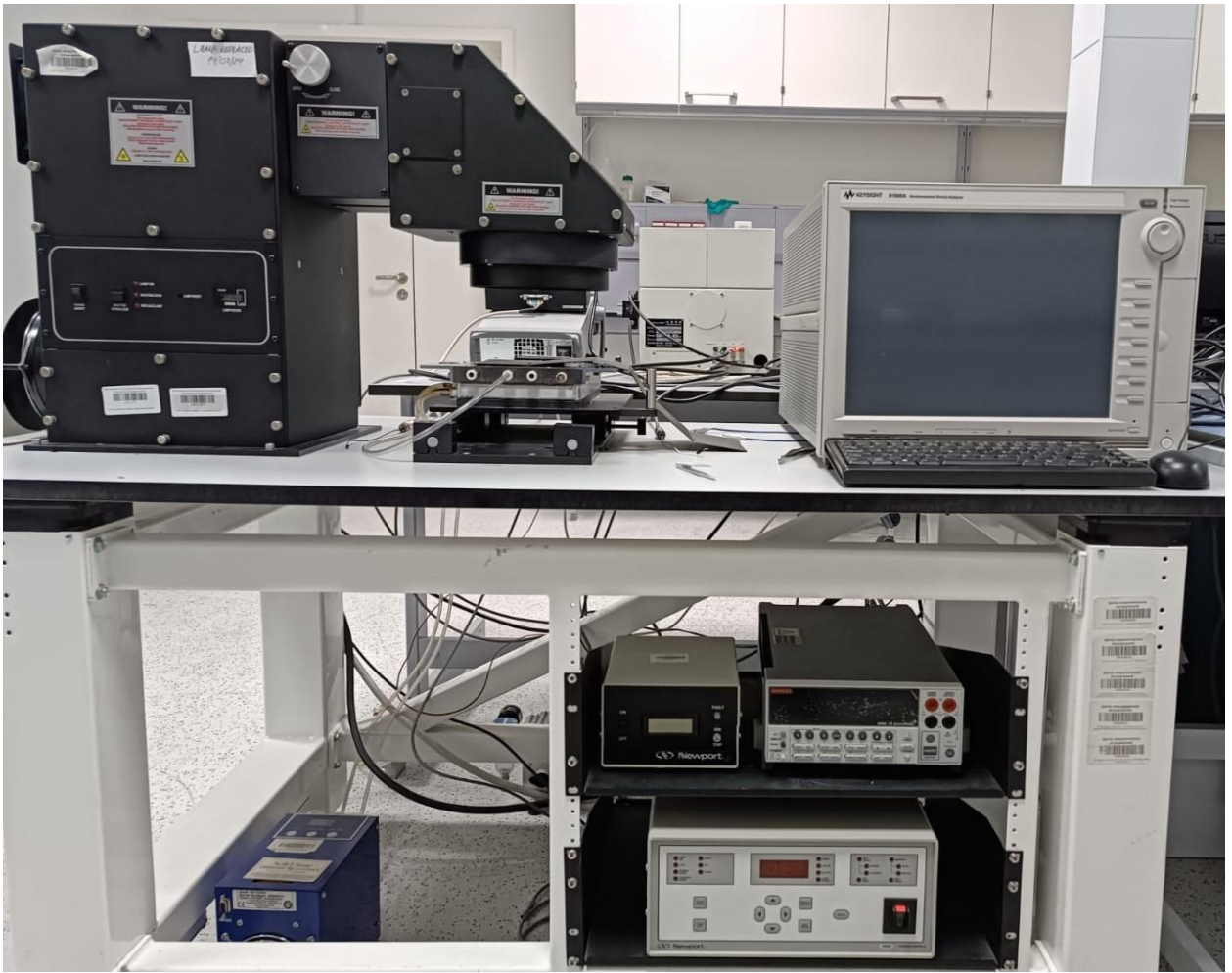
Figure 3.9: Solar simulator and the light source used for the characterization of PSCs fabricated in the presented thesis
