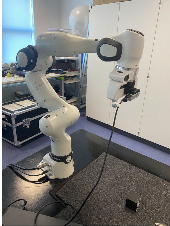
Figure 4-1: Robot with RGB-D camera mounted on a wrist.
