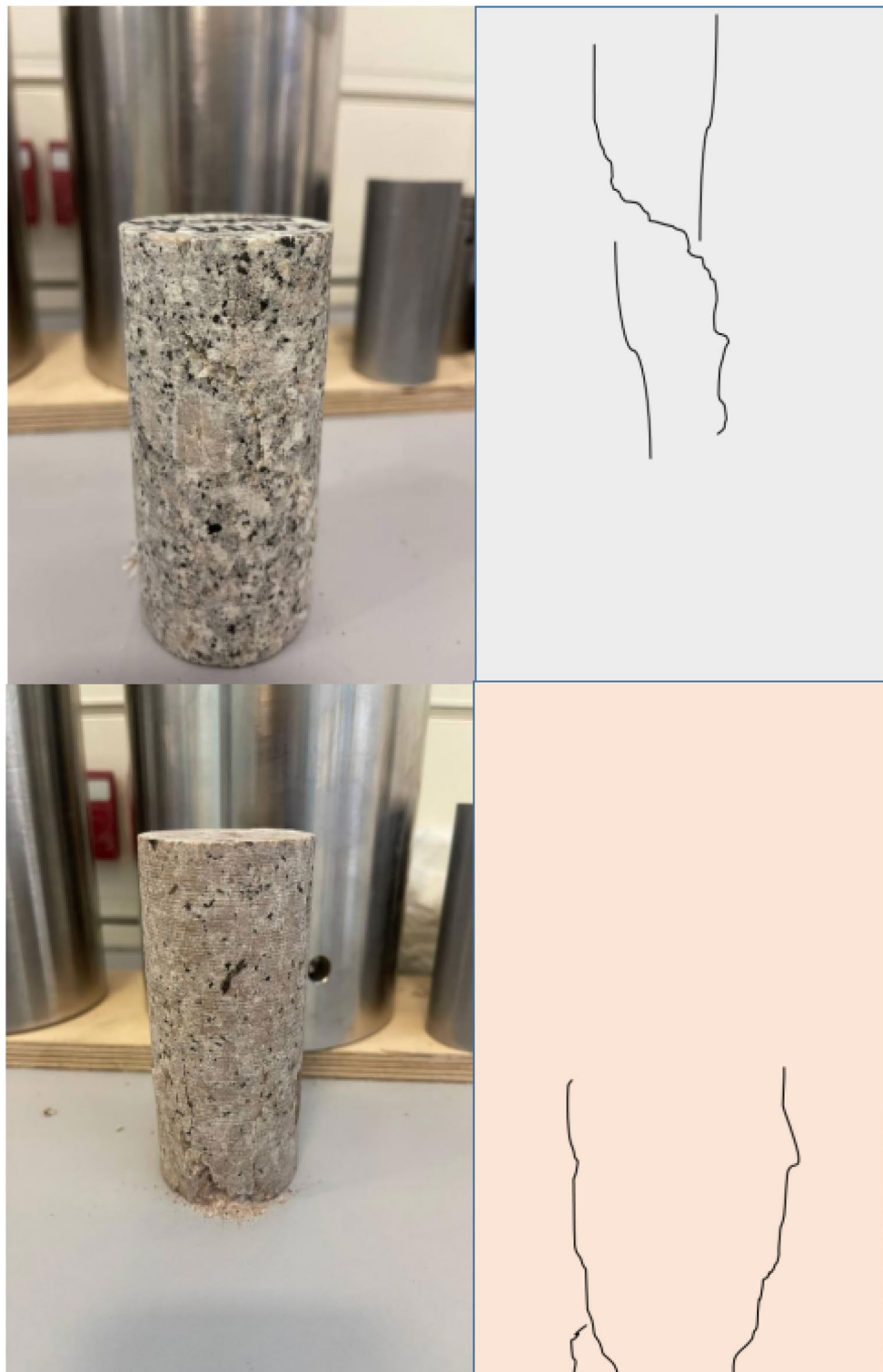
Figure 14. Specimens after compression tests with FT and FTC process after 300 °C and LN 2 treatment.
