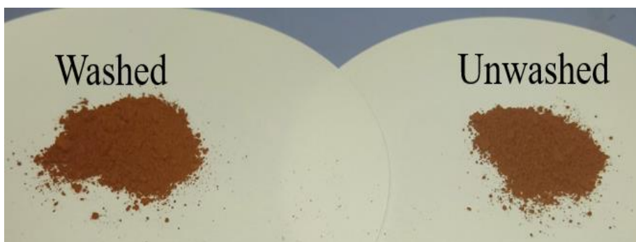
Figure 14. Comparison of washed and unwashed red mud samples after drying at 105 °C.
