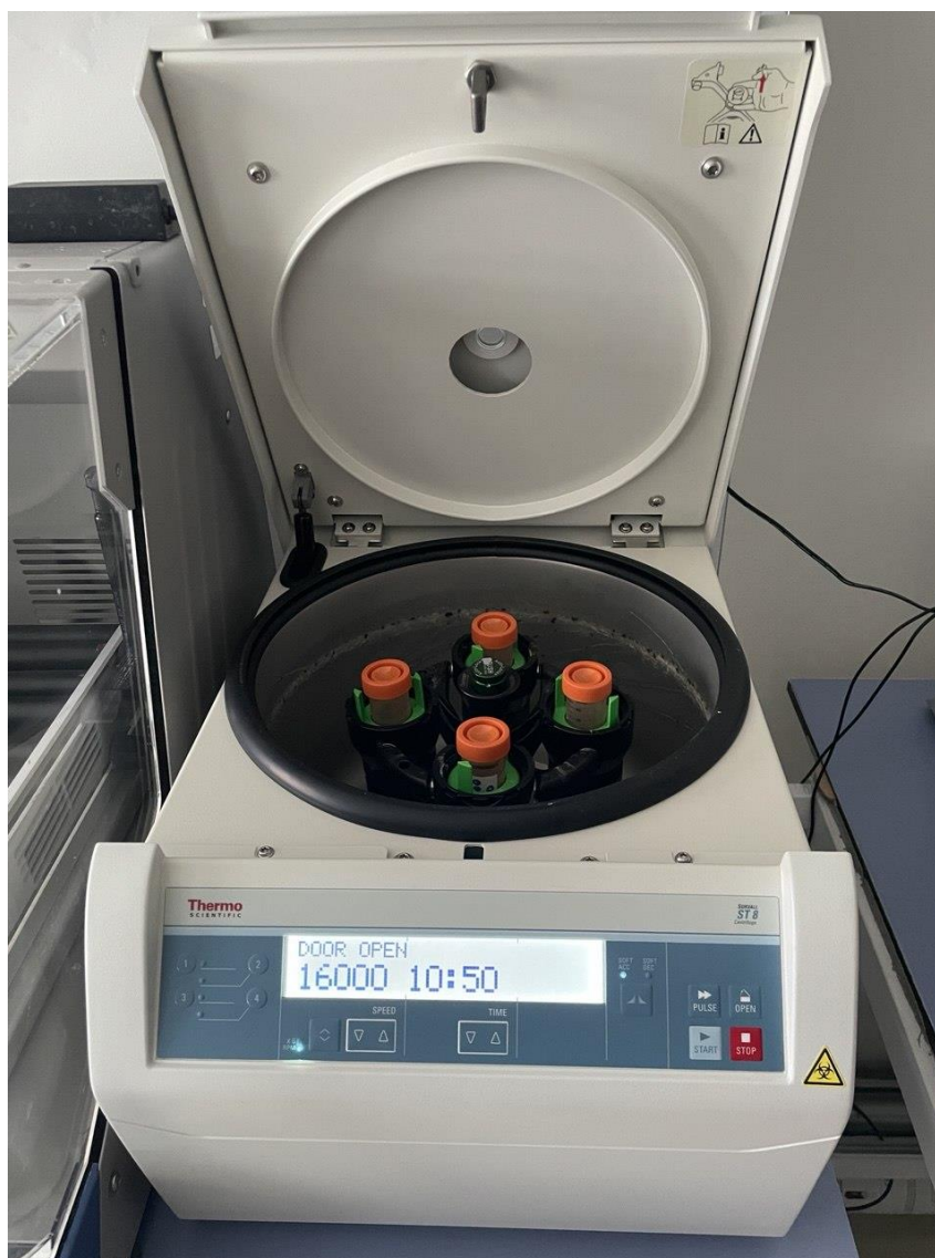
Figure 25. Centrifugation step used for solid-liquid separation of leachate samples prior to ICP-OES analysis.
