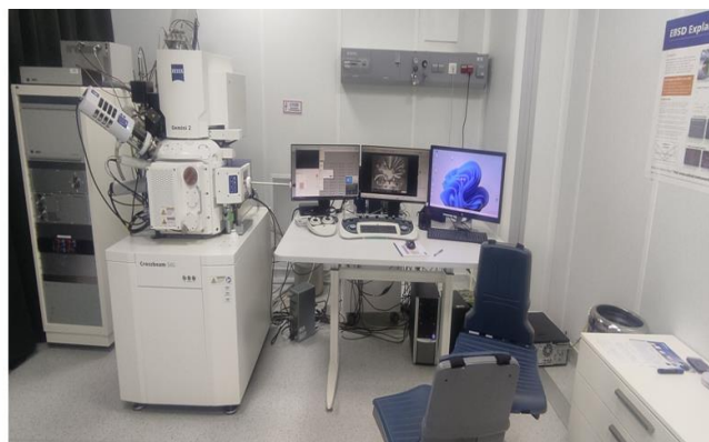
Figure 16. Zeiss Crossbeam 540 SEM-EDS (schematic (left) and laboratory setup (right)).
