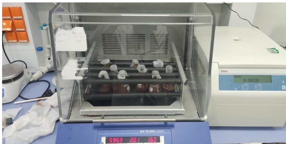
Figure 24. Laboratory orbital shaking incubator used for controlled chemical leaching experiments at 90 °C with regulated agitation speed.
