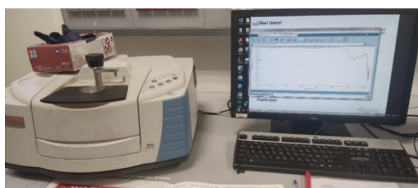
Figure 17. ATR-FTIR spectrometer (Thermo Scientific Nicolet iS12) and schematic of the FTIR measurement process.
