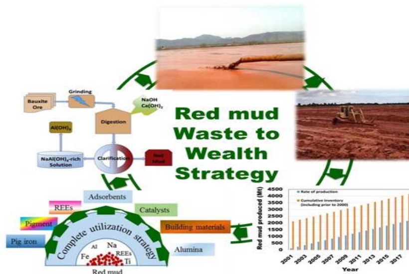
Figure 1. Conceptual illustration of red mud valorization within a circular economy, highlighting its conversion into valuable products and metals (Fe, Al, Ti, REEs) to support sustainable resource utilization (Swain, Akcil, and Lee 2022).
