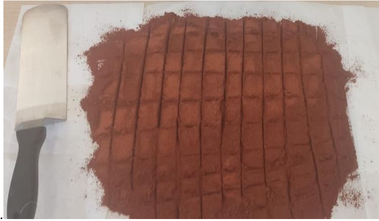
Figure 12. Powdered KRM sample after grinding and sieving, showing uniform particle size.
