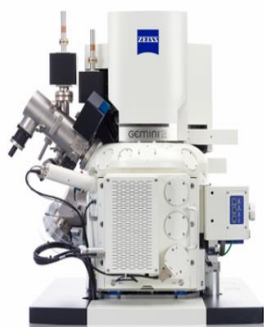
Figure 16. Zeiss Crossbeam 540 SEM-EDS (schematic (left) and laboratory setup (right)).
