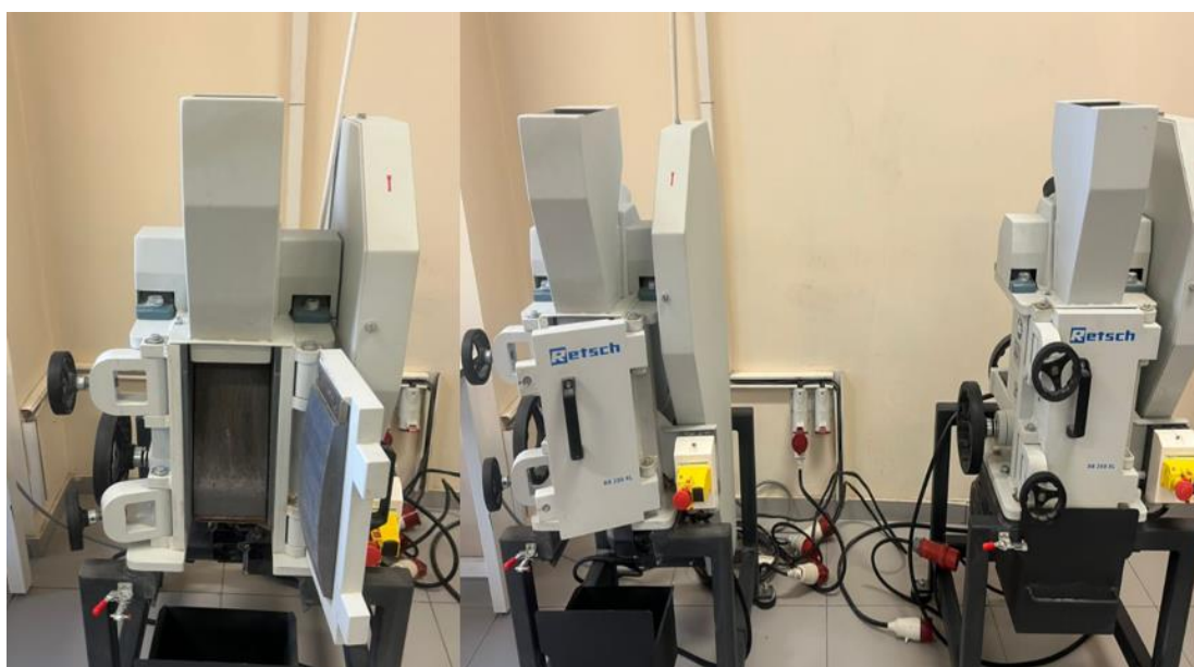
Figure 9. Jaw crusher used for comminution of KRM sample.
