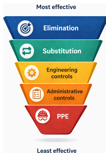
Figure 6.7.1 Hierarchy of Controls
