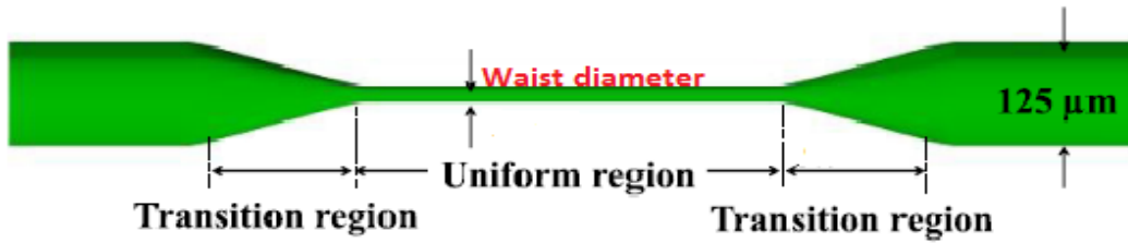
Figure 2.3: Fiber Optic Sensor Configuration
