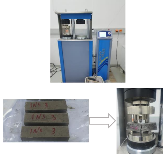
Figure 3.13. Flexural strength device and samples before and after testing
