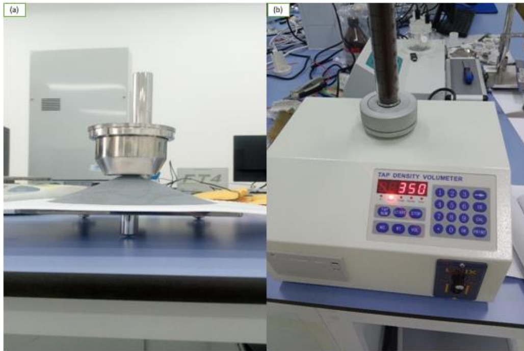
Figure 12. (a) Angle of repose determination using Hall flowmeter set-up (b) Tap density determination
