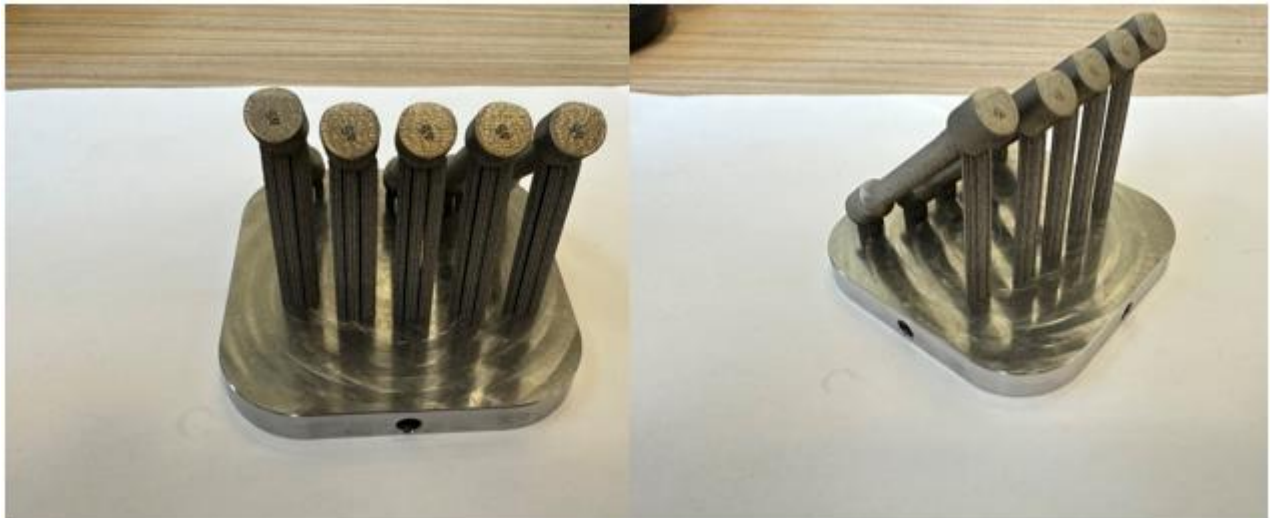
Figure 19. Standard tensile sample printed parts
