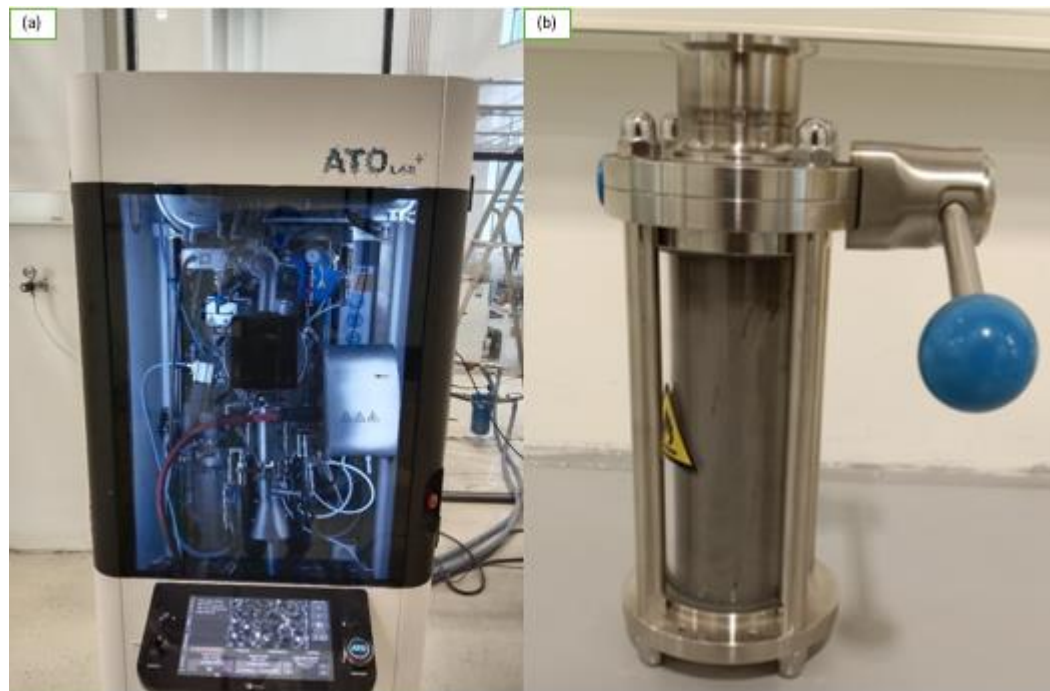
Figure 5. (a) Ultrasonic atomizer (b) Powder container
