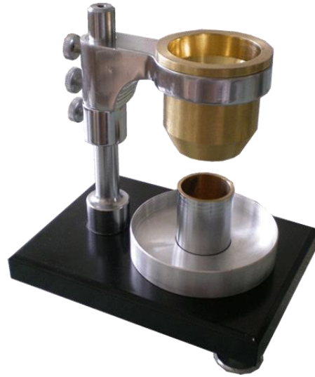
Figure 13. Hall flowmeter setup for flowrate determination
