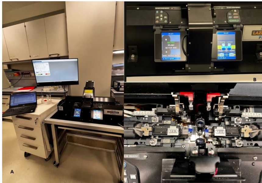
Figure 3. Fujikura LZM-100 machine (A) with interaction window (B) and single mode fiber placing area (C).
