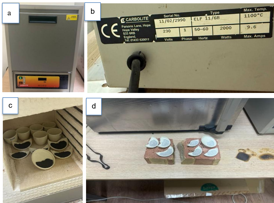
Figure 4. General view of Molodezhny coal mine: a) general view on the furnace b) Muffle furnace part number and model. c) coal sample in the muffle furnace d) high-temperature ash
